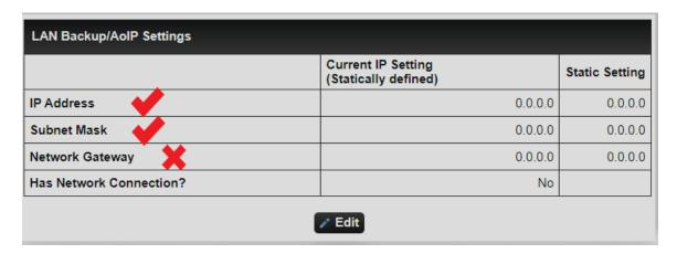
Once configured and after the Ethernet cable is connected into a Livewire Network switch the above Web page setup should show that the Audio Over IP interface has connection, 'HAS NETWORK CONNECTION?' > Yes. You can click the 'Refresh data' button to show Connection status if cable was installed after the setup. **Note: This connection status is only for the physical Ethernet NIC port.**
